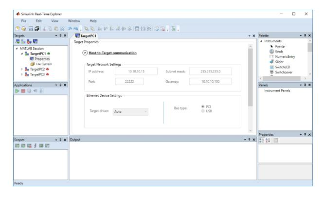
**Note** Support for using ISA bus Ethernet cards to communicate between the development and target computers has ceased to function. Use PCI bus or USB bus Ethernet cards instead.
