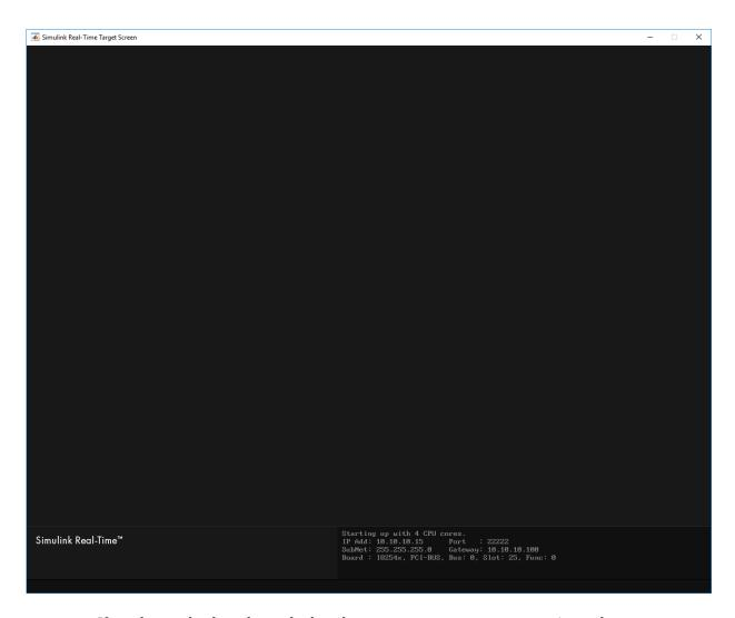
If you have a keyboard attached to the target computer, you can activate that keyboard by typing  ${f C}$ . Press the  ${f Page}$   ${f Up}$  and  ${f Page}$   ${f Down}$  keys to page up and down in the target computer monitor.
